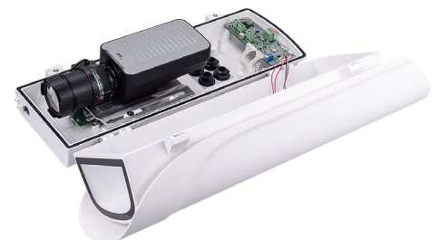
AXIS Q1635+ 8 – 80mm varifocal lens
